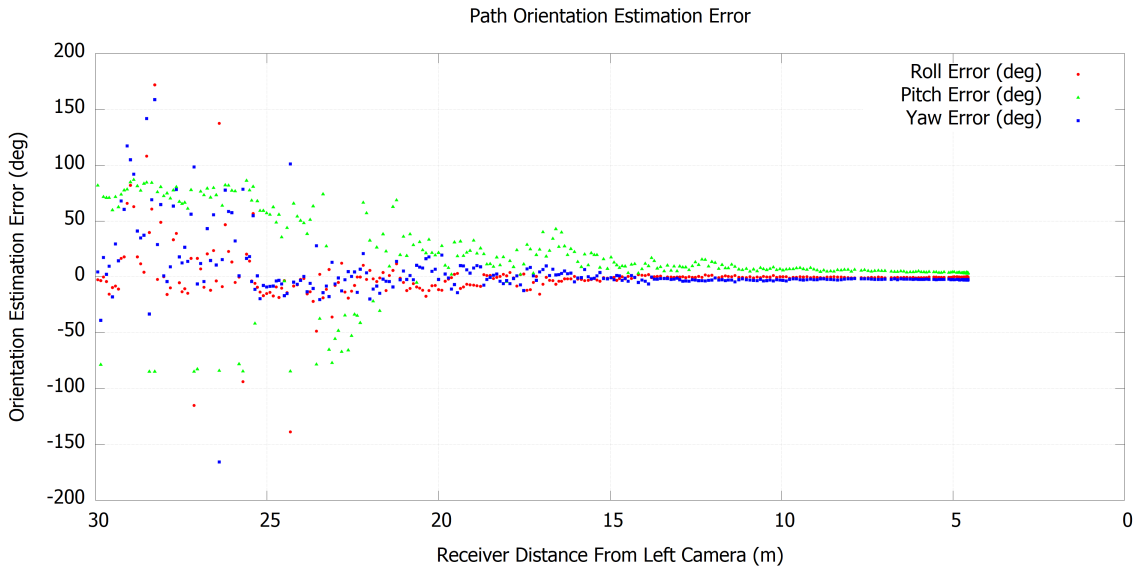
Figure 28. IR RPY Error for Test Run 1
