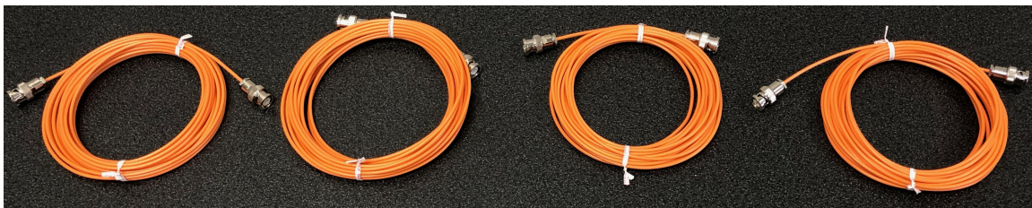
Figure 9. Coax Trigger Cables for Each Camera
