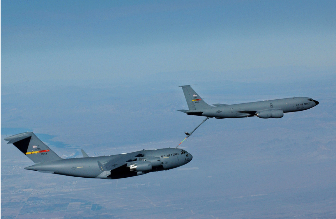
Figure 1. Cargo Plane Aerial Refueling via Boom Method from USAF Tanker [1]
